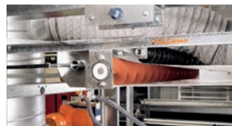
Manure belt idler roller with cleaning auger (option), removes dust and feathers from the returning belt
