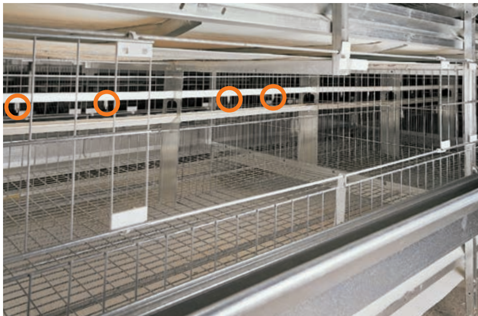
Grow tier UV-S 630 – four stainless steel nipples provide the birds with fresh water
